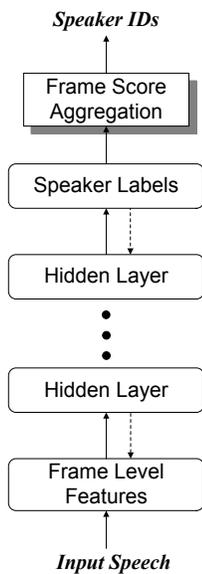
Figure 1. Schematic diagram of the proposed DNN based cochannel SID system
