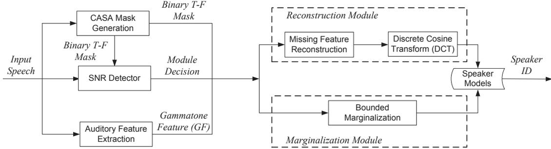
Figure 1. Schematic diagram of a CASA-based robust speaker identification system.
