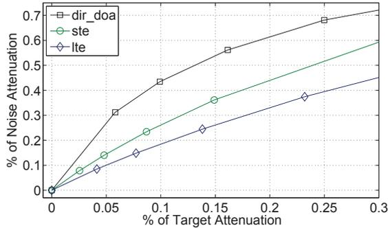
Fig. 1. Percentage of target attenuation versus noise attenuation as the parameter  $\beta$  is varied for 3 post-filter methods.
