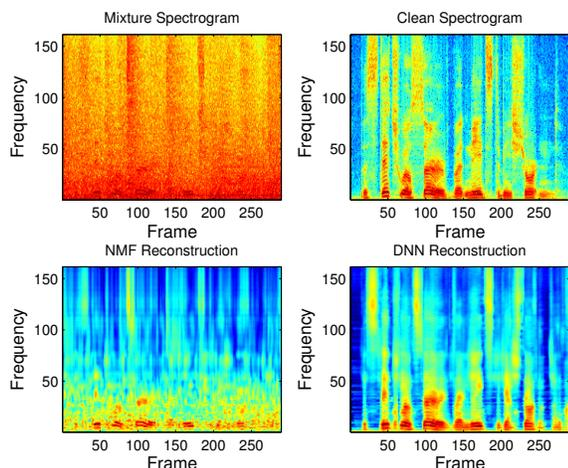
**Fig. 2.** Spectrogram reconstruction of a -5 dB mixture (factory noise). The DNN is trained to estimate the weights of the spectrogram bases learned by an NMF.
