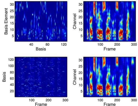
**Fig. 1.** A compositional model of the square-root IRM. Top left: 128 learned bases by training an NMF on square-root IRM (sliding window of 5 frames). Top right: the square-root IRM of a noisy mixture at -5 dB. Bottom left: basis weights inferred by the NMF. Bottom right: the reconstructed square-root IRM by using the resulting weights and bases.
