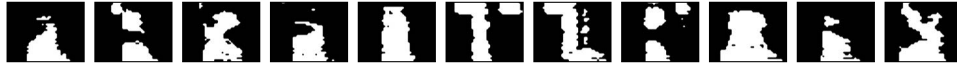
Fig. 1. Typical ideal binary masks of isolated digit utterances 1–9, ‘oh’ and ‘zero’, ordered from left to right. In the figure, a white pixel indicates 1 and black pixel 0.
