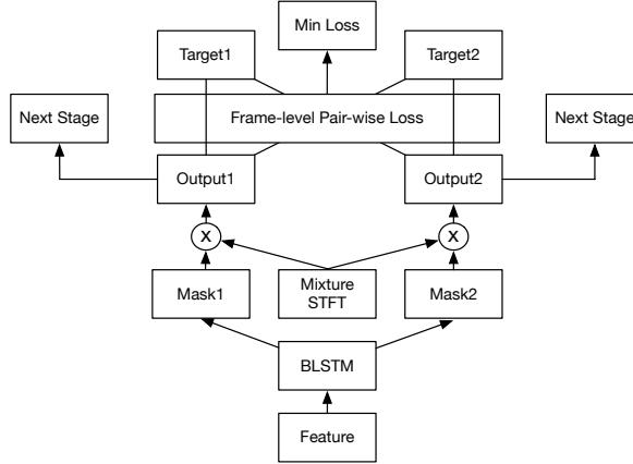
**Fig. 1:** Diagram of the simultaneous grouping stage.
