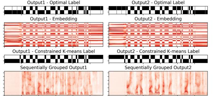
**Fig. 4:** Results of the sequential grouping stage for the same male-male test mixture as in Fig. 3. All horizontal axes correspond to time. First row: optimal speaker assignment label of the two output layers. Second row: estimated embedding vectors of the two output layers. Third row: estimated speaker assignment label after constrained K-means clustering. Last row: sequentially grouped outputs using K-means labels.
