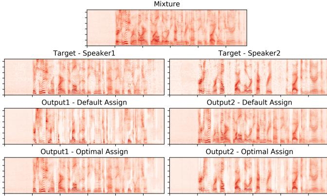
**Fig. 3:** Results of the simultaneous grouping stage for a male-male test mixture. First row: magnitude STFT of the mixture. Second row: magnitude STFT of the two targets. Third row: two outputs with the default speaker assignment. Last row: two outputs with the optimal speaker assignment.
