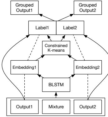
**Fig. 2:** Diagram of the sequential grouping stage.
