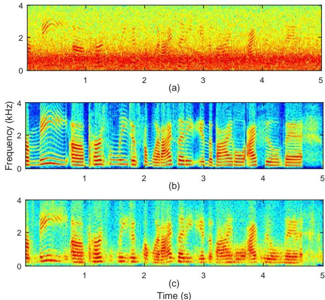
**Fig. 2:** Speech separation illustration. (a) Power spectrogram of a speech utterance mixed with SSN at -5 dB SNR, (b) Power spectrogram of the original speech signal, and (c) Power spectrogram of the separated speech signal.
