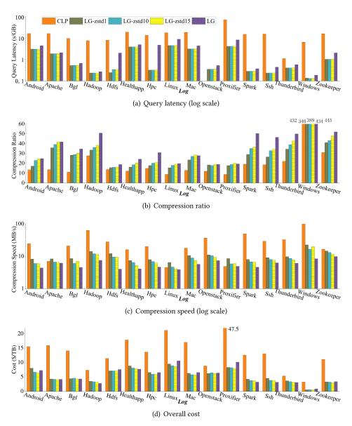
Fig. 17. Query latency, compression ratio, compression speed, and overall cost of different packing methods.
