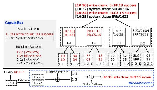
Fig. 1. Fine-grained storage format and reconstruction process. The log block shown above is structurized as four variable vectors in two groups, and these vectors are further structurized as eight Capsules. A user query (e.g., "bk.FF.") first locates the hit positions and then reconstructs the original log entry.
