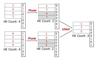
Fig. 6. Basic operations on the Indexed Bitmap structure. Two Indexed Bitmaps are first pruned to narrow down each hit scope and are finally united as one Indexed Bitmap.
