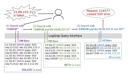
Fig. 2. A usage example of LogGrep to trace root cause by debugging interactively.
