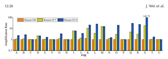
Fig. 16. The effect of partial reconstruction to the amplification rate on production logs (log scale).
