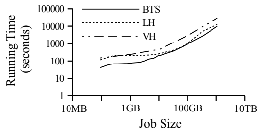
Fig. 10: Comparison of BTS to VH and LH in terms of running time. Note log-log scale.
