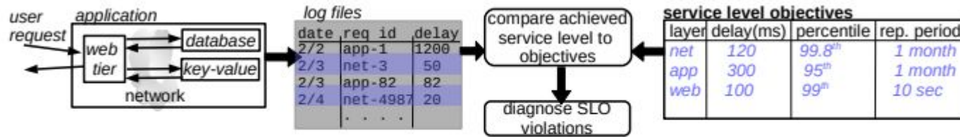
Fig. 2. The structure of SLO performance goals (right) reflects the workflow of cloud services (left). Logs highlighted in blue are aggregated during a reporting period.
