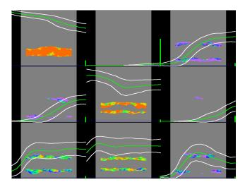
Fig. 4. A cluster spreadsheet featuring the mix fraction variable of a 122 time step combustion data set. The spreadsheet is only showing clusters for 15.25 time step trends for the low wavelet coefficients. The thumbnail of the data points for each cluster is rendered, and the centroid time curve of the data points is rendered on top in a green curve.
