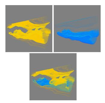
Fig. 15. The left image shows a temporal cluster from the OH variable of the combustion data. The right image shows a temporal cluster from the mix fraction variable. The bottom image is a projection or combination of the two variables in the same space to show coincidence and overlap. The bottom volumetric region the two clusters from the two variables overlap with each other and share similar structural features.
