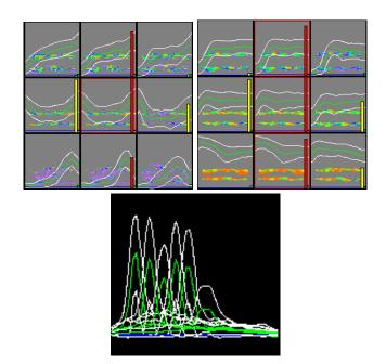
Fig. 14. The left image is a portion of spreadsheet of the OH variable. The right is a portion of spreadsheet of the mix fraction variable over time. The bottom image is an overlay cell from the  $\chi$  variable, showing a value moving through space over time.
