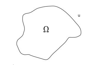
Dirichlet conditions if  $u\Big|_{\partial\Omega}$  is specified Neumann conditions if  $\frac{\partial u}{\partial n}\Big|_{\partial\Omega}$  is specified Robin conditions if  $a\frac{\partial u}{\partial n} + bu\Big|_{\partial\Omega}$  is specified
