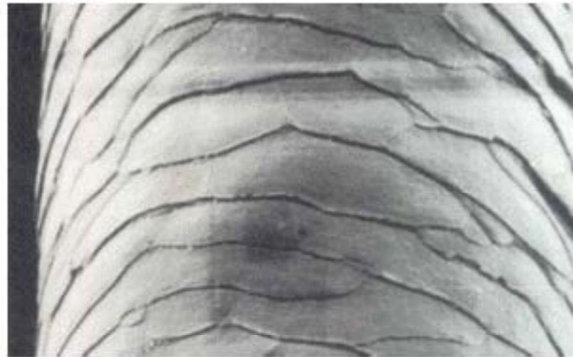
Fig. 11. An electron micrograph of a hair fiber that shows the structure of the outer cuticle surface, which is composed of thin overlapping scales [4].
