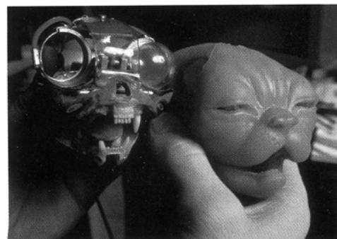
12.5.1 These two images illustrate the importance of animating the facial skin through the use of simulated bones, joints, and ligaments. On top, the mechanism of an animatronic cat's head built for a feature film appears alongside the skin that will eventually cover it. Below is a complex animatronic underskull for a feature film fantasy character. (Courtesy of Jim Henson's Creature Shop.)
