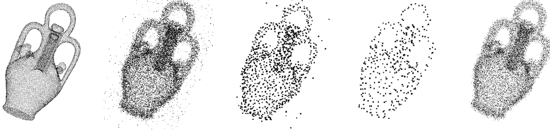
Figure 4: (a) – (d) show results of the Algorithm Declutter: (a) the ground truth, (b) the noisy input with 15K points with 1000 ambient noisy points, (c) the output of Algorithm Declutter when k = 9 , (d) the output of Algorithm Declutter when k = 30 . In (e), we show the output of Algorithm ParfreeDeclutter. As shown in Appendix E, algorithm ParfreeDeclutter can remove ambient noise for much sparser input samples with more noisy points.
