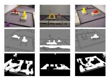
Figure 1. Top row: the layout of the BALL experiment. There are two large obstructions in the scene we wish to extract. Middle row: results of our method. Bottom row: cumulative background subtraction results on this sequence.
