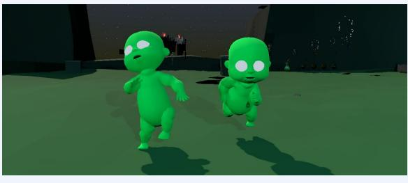
The ragdoll actually consists of two models: one that plays a predetermined animation and one that only moves based on a series of configuration joints. Each frame the joints on the physical model will apply forces to attempt to duplicate the transforms of the animated model. The movements of the physical model propels itself forward to match the input given by the player. The picture below shows the physical model on the left and the animated on the right.
