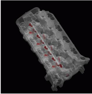
Figure 10: The thickness shell of the Engine, at 10mm thickness and 0.1mm error tolerance. This image can be rendered at 30frames/sec.
