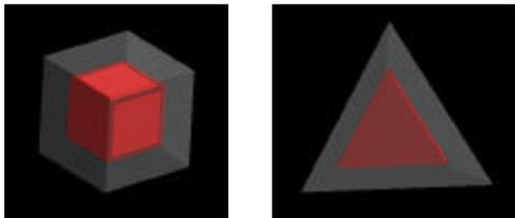
Figure 6: A sample model cube and a sample model of a tetrahedral cell, with the surface mesh shown in semi-transparency, and the inner shell at a distance value that is half the size of the cube, shown in red.
