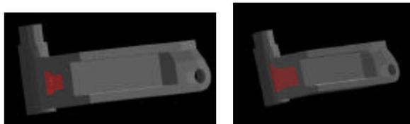
Figure 8: Results of a part design, Connector, with 327 triangles. The surface mesh is shown in semi-transparency, and the inner distance shell picked are at thickness 0.6 and 0.5, both at an accuracy of 1000th the size of the part's length. Picking a different initial resolution of CDFR, does not affect the final results, but results in different timings.
