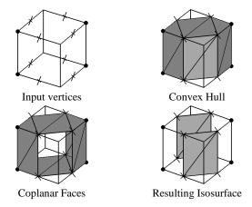
**Figure 1b.** Three-dimensional example of the algorithm. the boundary of the hypercube. This causes the removal of any facets, which share a vertex with the hypercube. The remaining (*d*-1) facets comprise the isosurface in the hypercube and are written into the lookup table. To generate the complete table, we repeat the above for each of the  $2^{2^d}$  possible cases.
