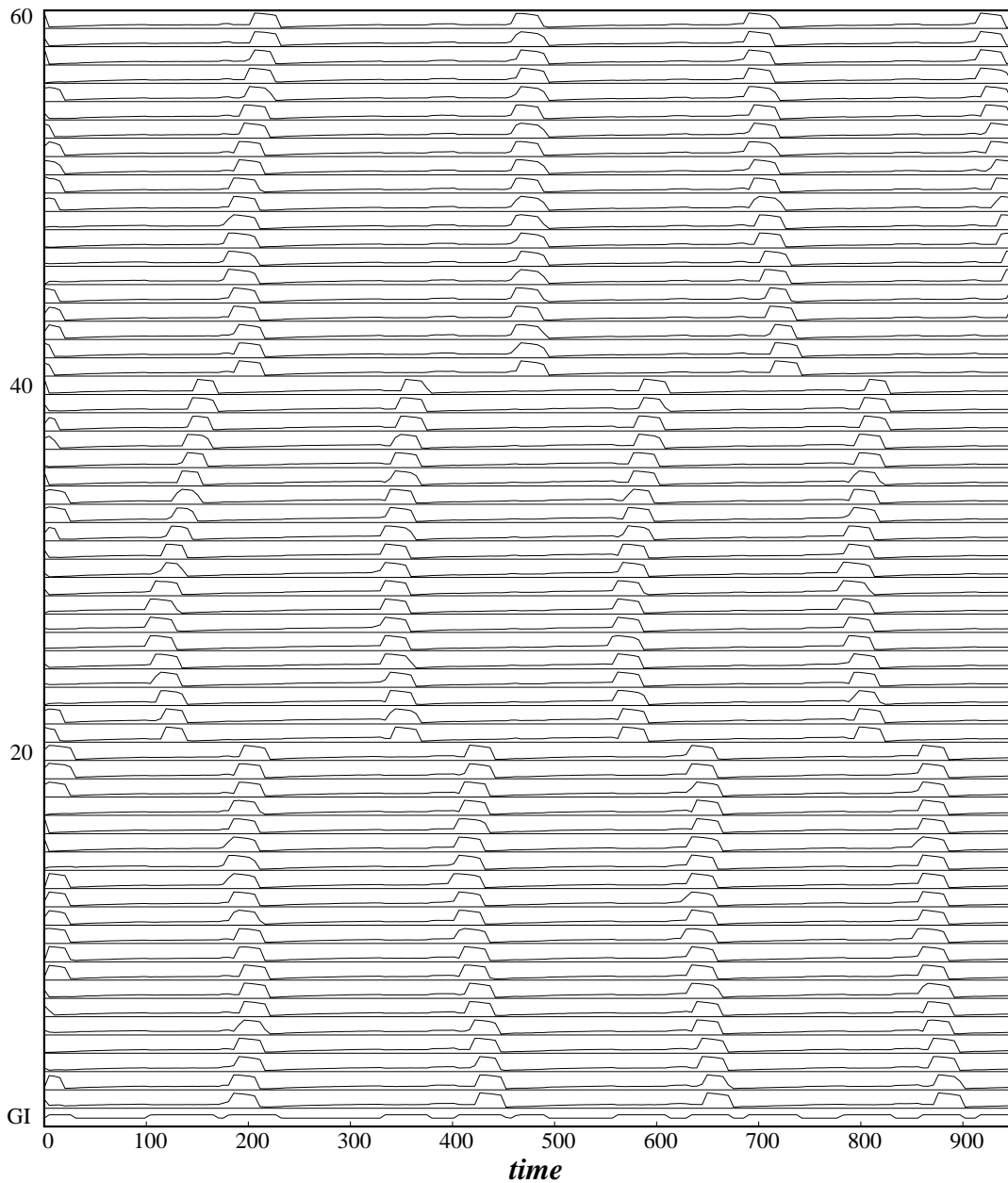
Figure 49. An example of LEGION dynamics with time delays in the coupling between oscillators. The temporal activity is displayed for 60 oscillators and GI. The activity of GI is displayed beneath the oscillators. The following parameter values are used: \gamma = 6 , \lambda = 3.95 , \alpha_R = 2 , \tau = 1 , \kappa = 500 , \beta = 1000 , \theta = -0.5 , and \varepsilon = 0.025 .
