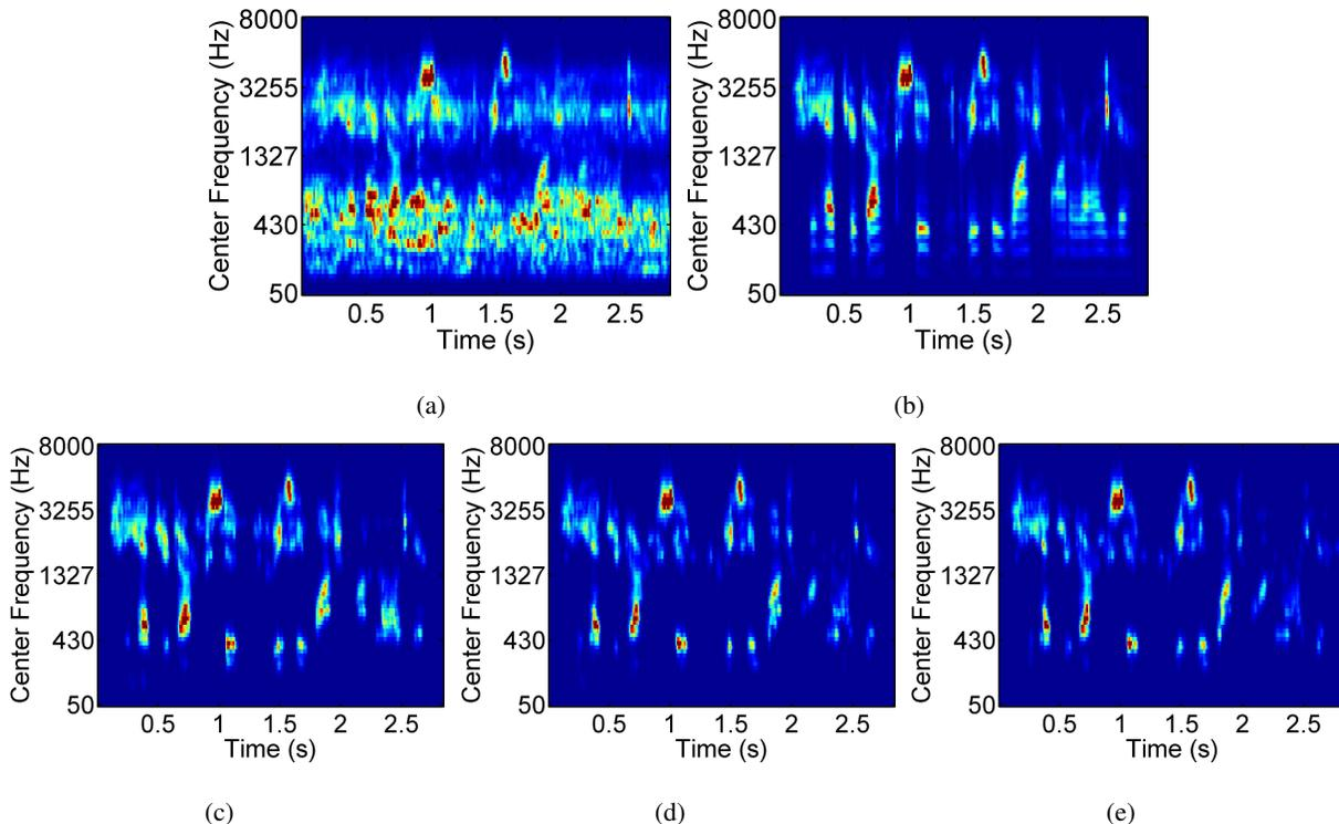
Fig. 3. Segregation illustration for a TIMIT utterance mixed with a babble noise at -5 dB. (a) Cochleagram of the mixture. (b) Cochleagram of the target utterance. (c) Cochleagram of separated speech with CCF+2D-ILD features. (d) Cochleagram of separated speech with ITD+2D-ILD features. (e) Cochleagram of separated speech with ITD+1D-ILD features.
