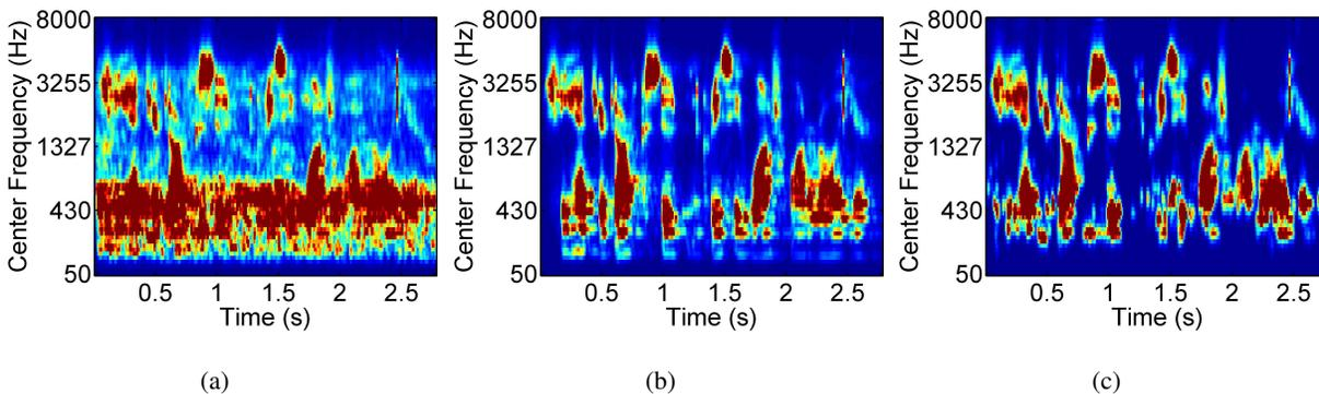
Fig. 10. Segregation illustration for a TIMIT utterance mixed with babble noise in Room C at 0-dB SNR. (a) Cochleagram of the reverberant mixture. (b) Cochleagram of the reverberant target utterance. (c) Cochleagram of separated speech.
