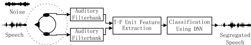
Fig. 1. Schematic diagram of the proposed binaural DNN classification system.
