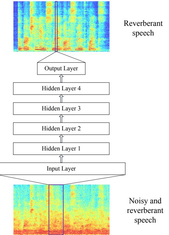
**Fig. 1.** DNN-based spectral mapping
