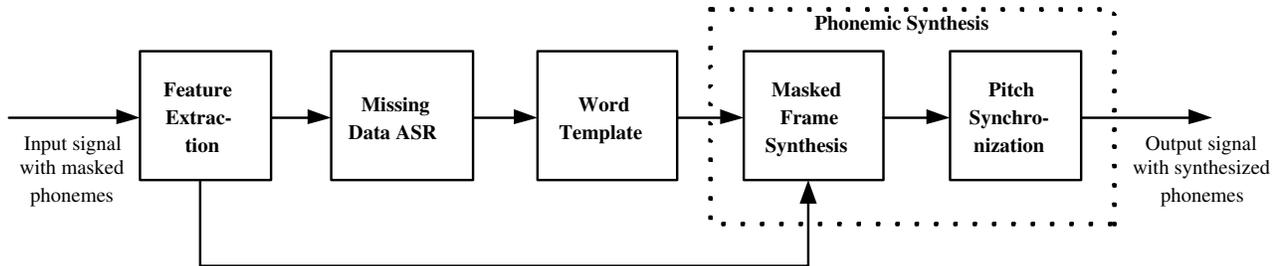
**Fig. 1.** Block Diagram of the proposed system. The input signal with masked phonemes is converted into the spectral domain and is fed to the missing data ASR, which activates trained word templates corresponding to the words whose phonemes are masked. The masked frames are synthesized by dynamically time warping the templates to the noisy words. These frames are then pitch synchronized with the rest of the utterance.
