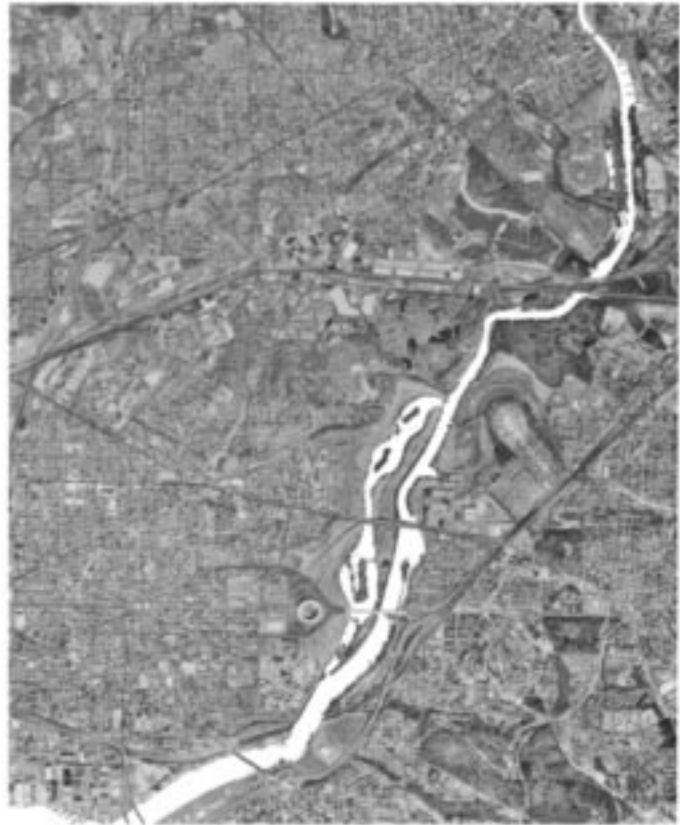
Fig. 2. Extracted hydrographic regions from the DOQQ image shown in Fig. 1. Hydrographic regions are marked as white and superimposed on the original image to show the accuracy of the extracted result. Here, W_z = 0.15 and \theta_p = 4000 . It takes about 100 min on an HP workstation to generate this result.
