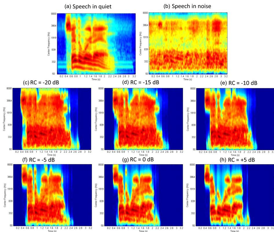
Fig. 2. (Color online) Spectrogram representations of, “Say the word *an*.” (a) In quiet and (b) mixed with noise from a busy cafeteria at  $-8$  dB SNR. Shown in (c)–(h) are the speech-plus-noise mixture in (b) after IBM processing to extract the target speech using six different RC values (RC = dB rel. to overall SNR).
