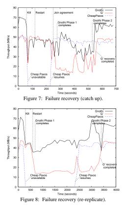
G' can also complete recovery at time 3400, but during this period, it can only service new requests at a rate of about 16 MB/s.
