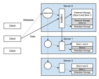
Figure 1: Data and metadata flow for a request to update a block in slice 1.
