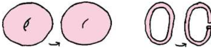
Figure 4: Two ways to remove a handle: left: collapsing the handle, right: pinching the Handle [Wood et al , “Removing Excess Topology From Isosurfaces”, 2004]
