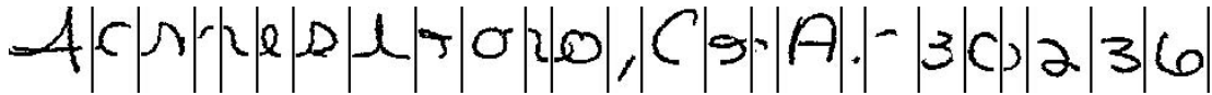
Figure 5.3: The result of over-segmentation: The graphemes obtained after over-segmentation of the address line shown in Figure 5.2 are shown separated by vertical lines.
