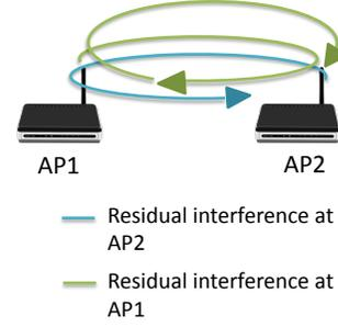
Figure 4: Looping of residual interference between the APs
