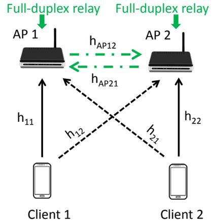
Figure 1: System model with 2 clients transmitting to 2 APs
