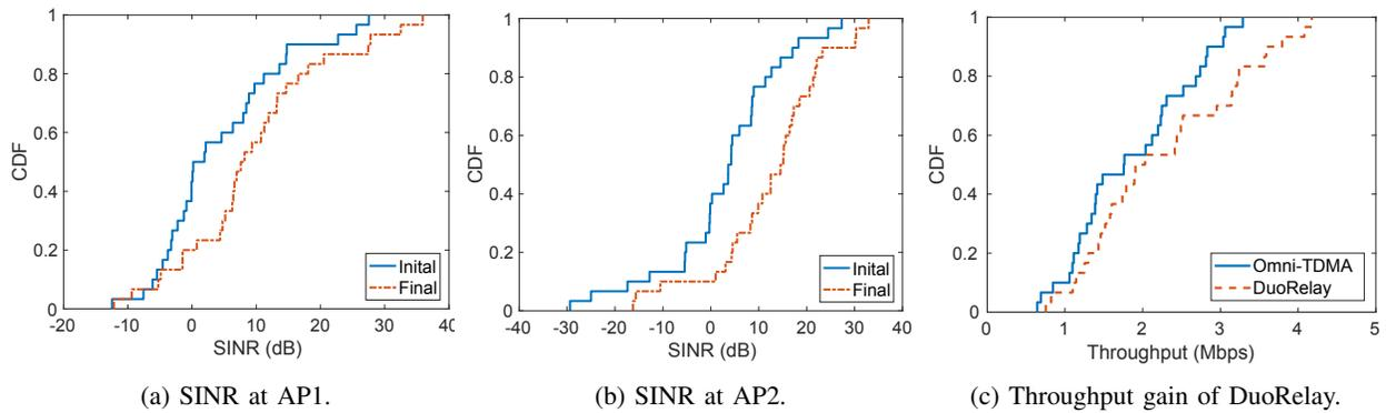
Figure 7: SINR performance and throughput of DuoRelay with interference looping.
