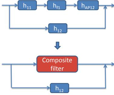
Figure 3: Equivalent filter-modeling of the relayed path
