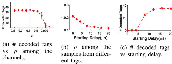
Fig. 5: # decoded tags vs channel and sample independence.
