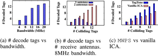
(a) # decode tags vs bandwidth. (b) # decode tags vs # receive antennas. (c) MWPS vs vanilla ICA.
