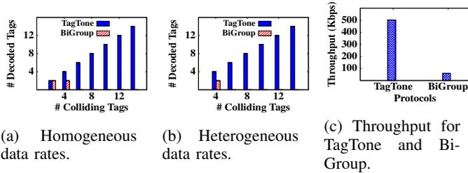
(a) Homogeneous data rates. (b) Heterogeneous data rates. (c) Throughput for TagTone and BiGroup.
