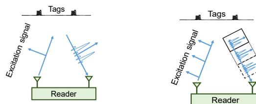
(a) Current protocols do not use the whole bandwidth because the excitation signal contains a single tone. (b) TagTone utilizes the whole bandwidth to decode a large number of tags.
