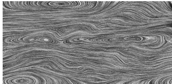
Figure 6: LIC image of the 573x288 ocean wind dataset in 1.9s, using convolution length 30.
