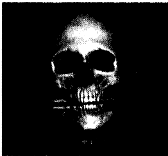
Figure 9. Volume rendering of 512 \times 512 \times 113 voxel CT dataset.
