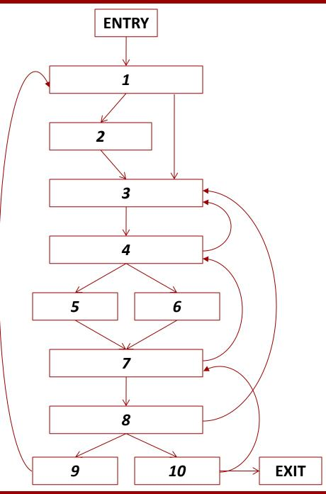
ENTRY *dom n* for any *n* 1 *dom n* for any *n* except ENTRY 2 does not dominate any other node 3 *dom* 3, 4, 5, 6, 7, 8, 9, 10, EXIT 4 *dom* 4, 5, 6, 7, 8, 9, 10, EXIT 5 does not dominate any other node 6 does not dominate any other node 7 *dom* 7, 8, 9, 10, EXIT 8 *dom* 8, 9, 10, EXIT 9 does not dominate any other node 10 *dom* 10, EXIT
