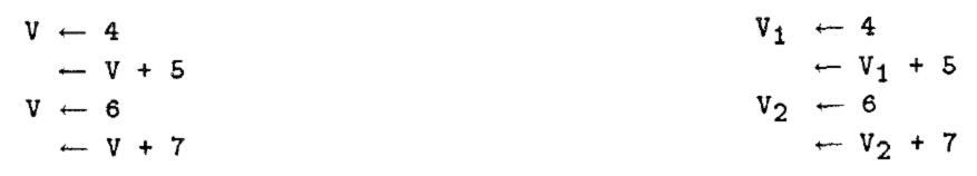
Fig. 2. Straight-line code and its single assignment version.
