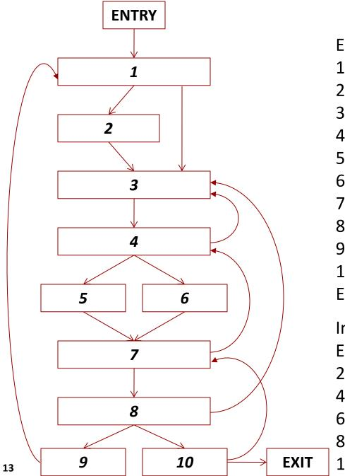
ENTRY does not post-dominate any other *n* 1 *pdom* ENTRY, 1, 9 2 does not post-dominate any other *n* 3 *pdom* ENTRY, 1, 2, 3, 9 4 pdom ENTRY, 1, 2, 3, 4, 9 5 does not post-dominate any other *n* 6 does not post-dominate any other *n* 7 pdom ENTRY, 1, 2, 3, 4, 5, 6, 7, 9 8 pdom ENTRY, 1, 2, 3, 4, 5, 6, 7, 8, 9 9 does not post-dominate any other *n* 10 *pdom* ENTRY, 1, 2, 3, 4, 5, 6, 7, 8, 9, 10 EXIT pdom n for any n
