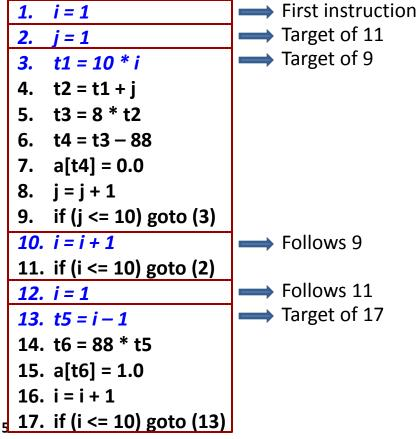
Note: this example sets array elements a[i][j] to 0.0, for 1 <= i,j <= 10 (instructions 1-11). It then sets a[i][i] to 1.0, for 1 <= i <= 10 (instructions 12-17). The array accesses in instructions 7 and 15 are done with offsets computed as described in Section 6.4.3, assuming row-major order, 8byte array elements, and array indexing that starts from 1, not from 0.
