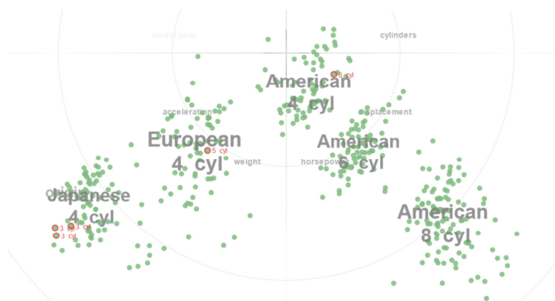
Figure 1: Just-in-Time Descriptive Analytics can automatically identify and annotate visual features (e.g. clusters, outliers, and trends) describing their semantics as users interact with visualizations by performing statistical computation at run-time. Shown above are about 400 cars, shown as dots, representing dimensions such as mpg, weight, horsepower, and origin. Five clusters are detected and annotated automatically with descriptive labels (e.g. “European, 4 cyl.”) distinguishing their semantics from others. Within each cluster outliers (encircled in red) are also detected and labeled automatically (e.g. “3 cyl”). Looking at these visualizations users can easily understand structure of the data, i.e. what each cluster represents semantically and how data is distributed across several clusters, and build a qualitative mental model.
