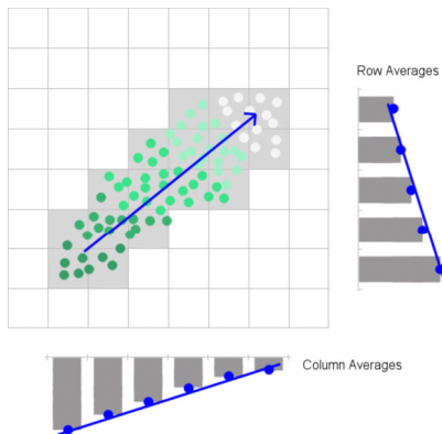
Figure 7: Directional trend algorithm examines vertical and horizontal average values for each dimension in each row and column of a cluster, and tries to fit them to a line. If the standard error between actual and estimated values is low and slope is above a threshold it is considered that there is a directional trend.
