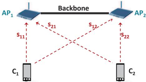
Figure 1: A  $2 \times 2$  network with 2 clients and 2 APs which are connected through the backbone network. The weight ( $s_{ij}$ ) of the dotted line is the received signal strength (RSS) at  $AP_j$  for transmission from  $C_i$  in *Watts*.
