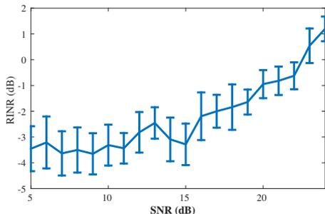
Figure 6: The residual interference to noise ratio (RINR) under different SNR conditions with 20 MHz bandwidth.
