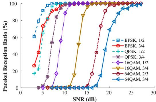
Figure 5: The SNR and Packet Reception Ratio of different modulation and coding schemes used in our evaluations.
