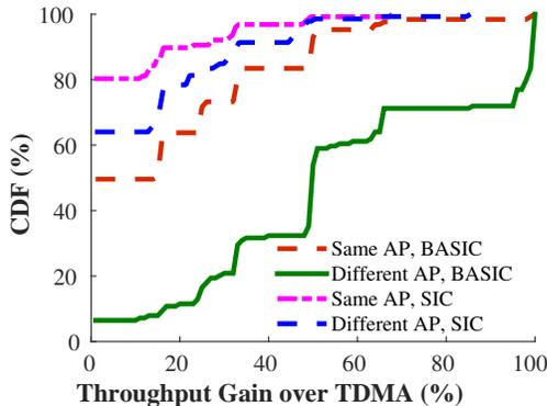
Figure 8: The throughput gain distribution of BASIC and SIC over TDMA in a  $2 \times 2$  testbed.
