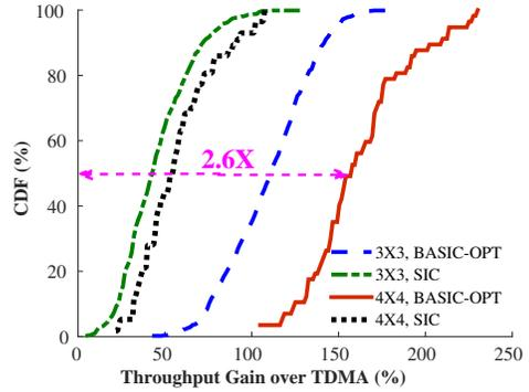
(b) Capacity gain over TDMA in  $3 \times 3$  and  $4 \times 4$  networks. For BASIC-OPT, the median gain of  $3 \times 3$  networks is 110% and the median gain of  $4 \times 4$  networks is 156%. For SIC, the median gain is 42% and 54%, respectively.
