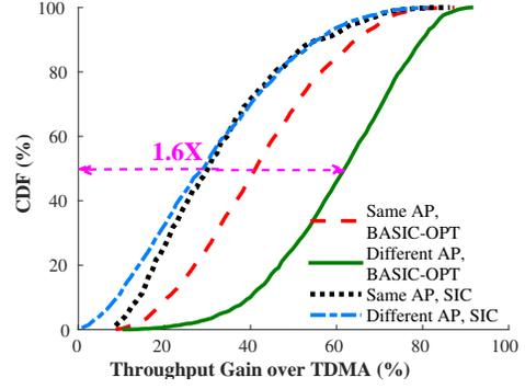
(a) Capacity gain over TDMA in  $2 \times 2$  networks. For BASIC-OPT, the median gain of 2 clients associated with the same AP is 41%, and the median gain for different association is 62%. For SIC, the median gain is about 29% in both cases.
