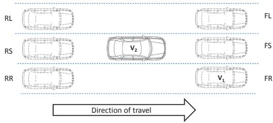
**Figure 1: Vehicle  $V_1$  can be in six different relative positions with respect to  $V_2$ : Front-Left, Front-Right, Front-Same, Front-Right, Rear-Left, Rear-Same and Rear-Right. Note that Front-Left, Front-Right, Rear-Left, and Rear-Right also include the cases that  $V_2$  is immediately to the left or right of  $V_1$ .**
