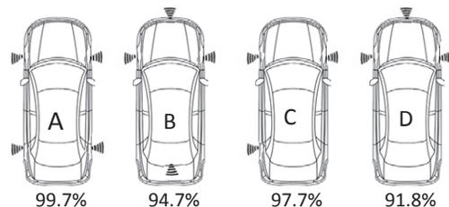
**Figure 5: Some combinations of placement of the wireless radios and the corresponding relative lane localization accuracy. A and B have four radios attached while C and D have 3 radios. The first classifier from configuration A has the highest prediction accuracy.**
