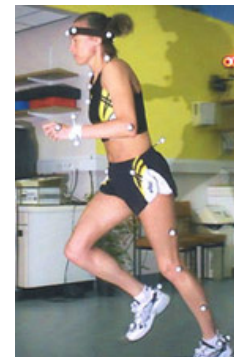
Reflective-marker system from Vicon
