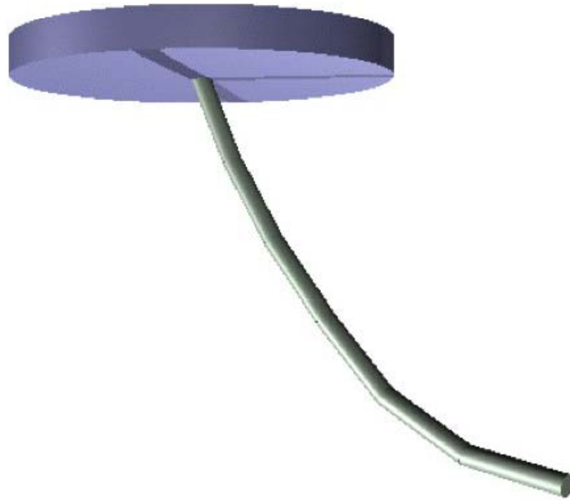
Figure 7: Simple multi-body pendulum made of six sticks.
