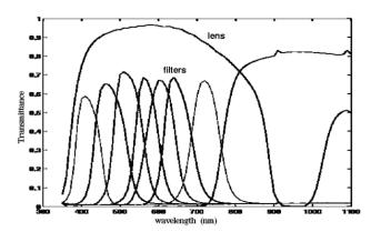
Figure 6: Spectral transmittance of filters used in spectral image reconstruction
