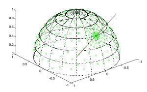
**Figure 9:** Sampling positions of BRDF measurements on the hemisphere above the sample surface. The solid line indicates the specular reflection direction.
