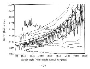
suring four two-inch diameter samples of a white diffuse surface, a black diffuse surface, an industrial grade molybdenum mirror and an aluminum mirror, both very smooth. The results showed an enormous range of deviation, confirming the difficulty of the task (Figure 10).
