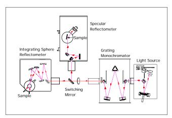
Figure 12: Schematics of equipment for measuring the diffuse and specular reflectances.
