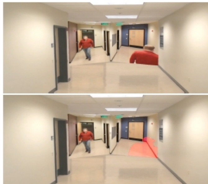
Figure 15 Illustration of near clip plane simulation by background subtraction. The back of the subject is sampled by the video camera that is supposed to sample the right branch of the corridor ( top ). The back of the subject is erased using a background image of the right corridor acquired before the subject appeared ( bottom ).
