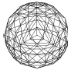
FIGURE 5.34 Sphere approximations using subdivision.
