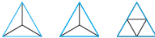
FIGURE 5.33 Subdivision of a triangle by (a) bisecting angles, (b) computing the centroid, and (c) bisecting sides.
