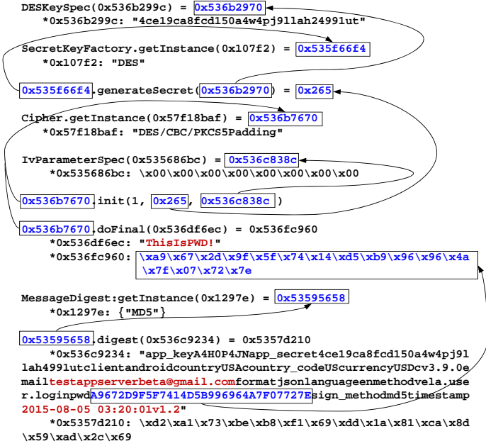
Fig. 3. Crypto API traces and the illustration of their arguments and return value dependencies of the miniintthebox App. Note that *addr denotes the content stored in that addr .
