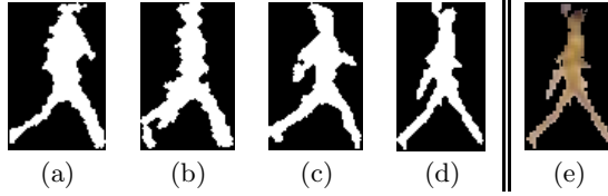
Figure 8: (a)-(d) Binary results for indoor sequences A-D and (e) Result of weighted color fusion for sequence D
