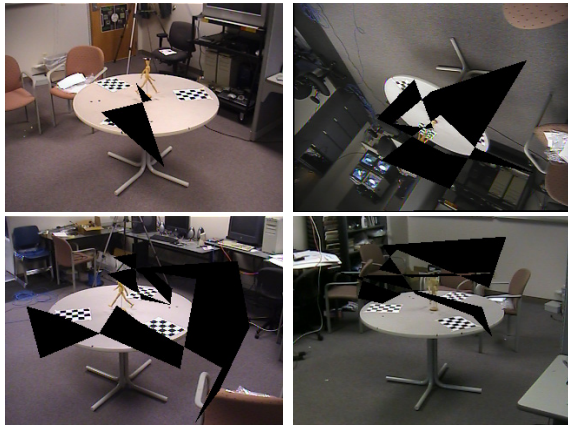
Figure 9: Manually created occlusions in the four camera views for an indoor sequence
