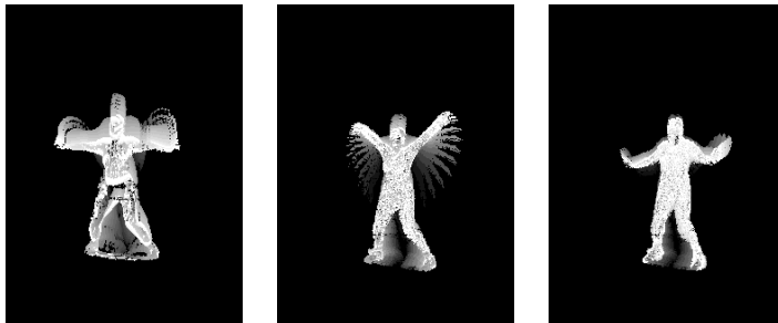
Figure 7. Example of error where failure is caused by both the inadequacy of using image differencing to estimate image motion and the lack of the variance data in the recognition procedure.
