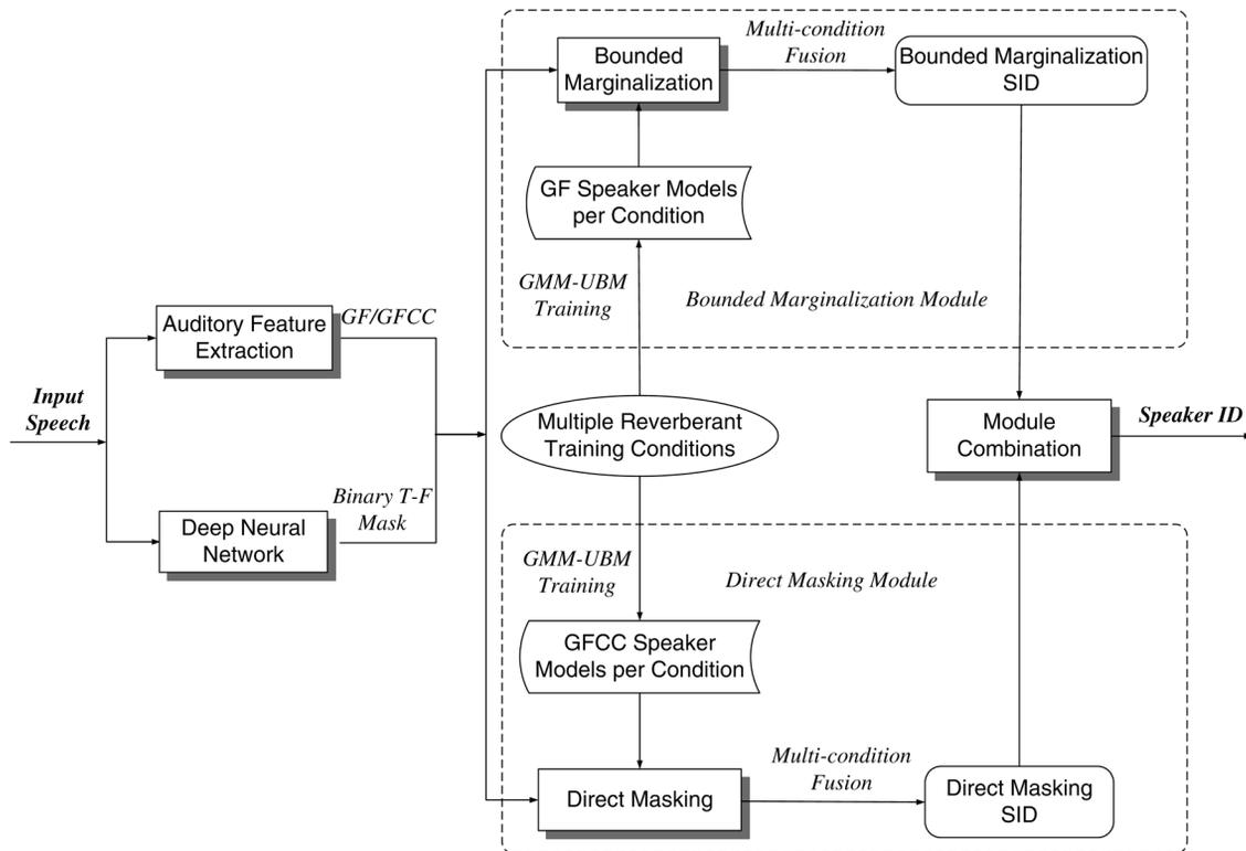
Fig. 1. Schematic diagram of the proposed speaker identification system.
