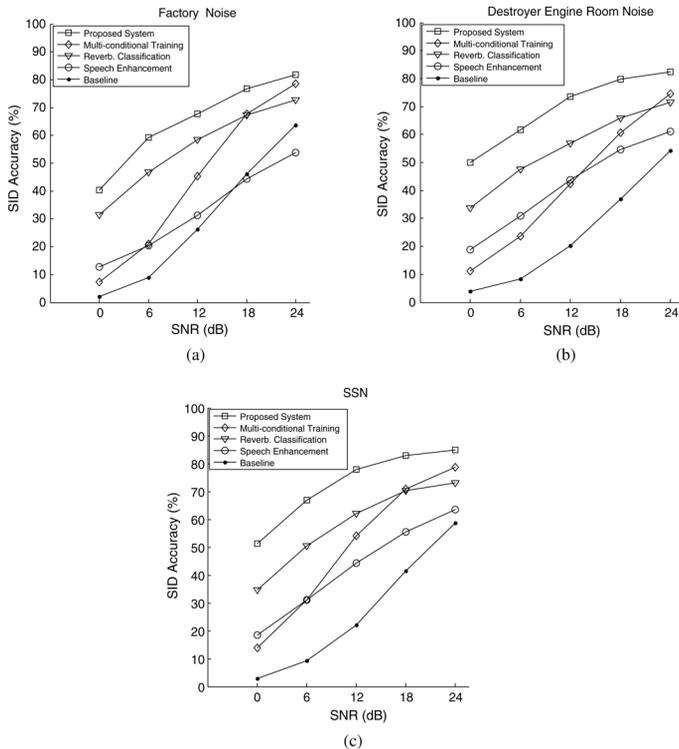
Fig. 4. SID comparisons of the proposed system with related systems under factory noise, destroyer engine room noise and speech shape noise using simulated RIRs.
