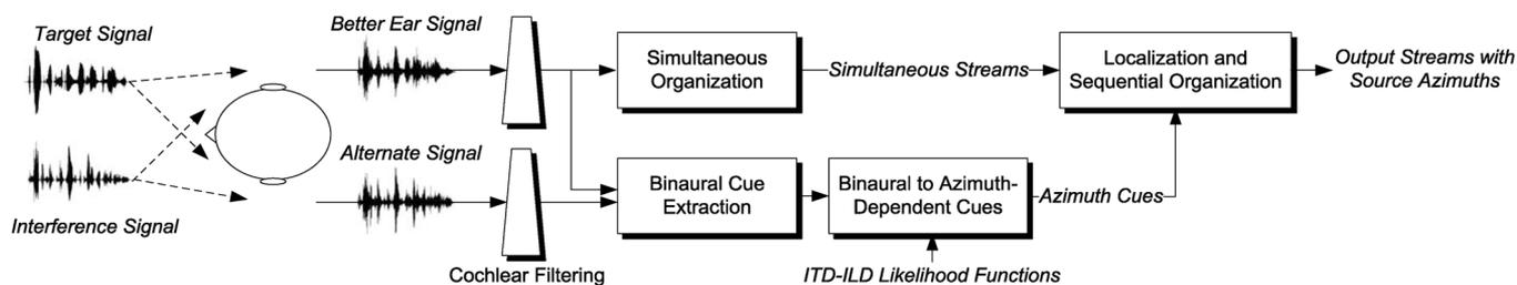
Fig. 1. Schematic diagram of the proposed system. Binaural recordings are fed as input to the system. Cochlear filtering is applied to both the left and right ear signals. Monaural processing generates simultaneous streams from the *Better Ear Signal*. Both signals are used to generate azimuth-dependent cues. Simultaneous streams and azimuth-dependent cues are combined in the final localization and sequential organization stage.
