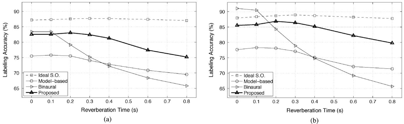
Fig. 5. Labeling accuracy of the proposed and comparison systems shown as a function of reverberation time for (a) two-talker and (b) three-talker mixtures.
