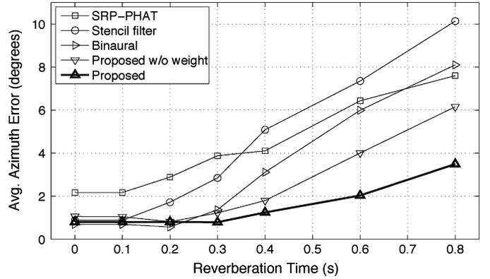
Fig. 4. Azimuth estimation error averaged over 200 two-talker mixtures, or 400 utterances, for various reverberation times. Results are shown using the proposed approach with and without cue weighting, and three alternative approaches.
