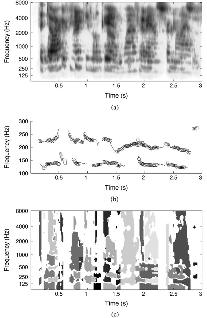
Fig. 2. Example of multi-pitch detection and simultaneous organization using the tandem algorithm. (a) Cochleagram of a two talker mixture. (b) Ground truth pitch points (solid lines) and detected pitches (circles and squares). Different pitch contours are shown by alternating between circles and squares. (c) Simultaneous streams corresponding to different pitch contours are shown with different gray levels.
