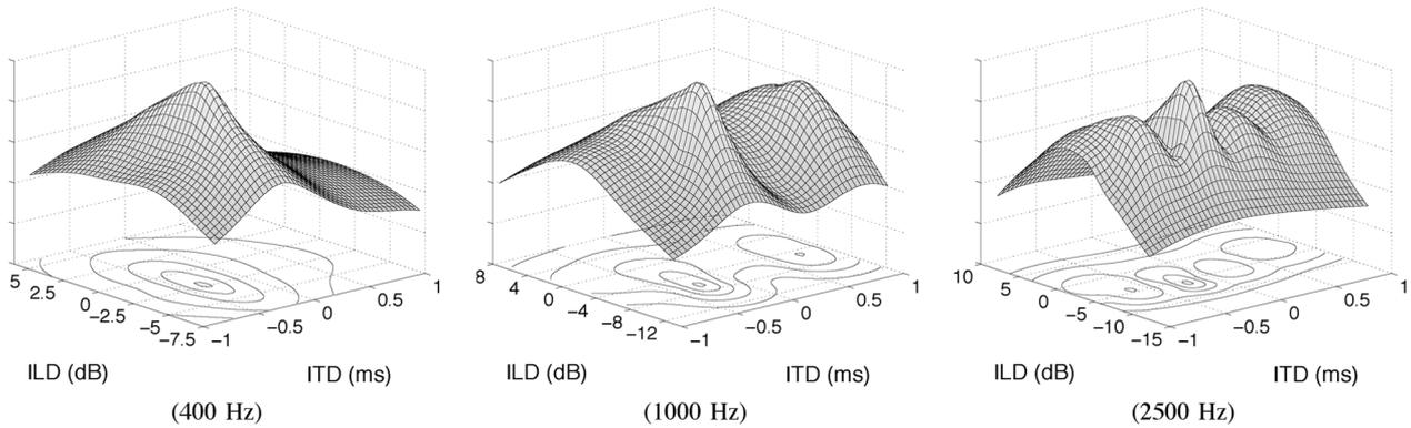
Fig. 3. Examples of ITD-ILD likelihood functions for azimuth  $25^\circ$  at frequencies of 400, 1000, and 2500 Hz. Each example shows the log-likelihood as a surface with projected contour plots that show cross sections of the function at equally spaced intervals.
