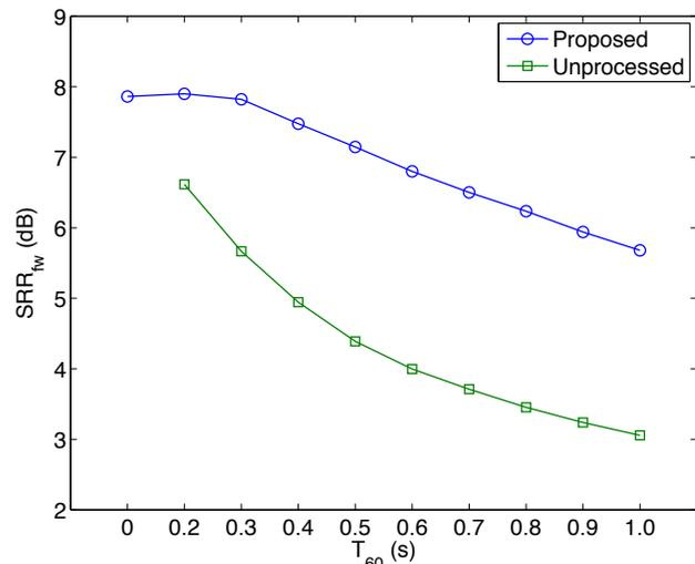
**Fig. 4:** Generalization results in different  $T_{60}$ . “Proposed” denotes the cochleagram mapping approach, and “Unprocessed” the results for original reverberant speech.
