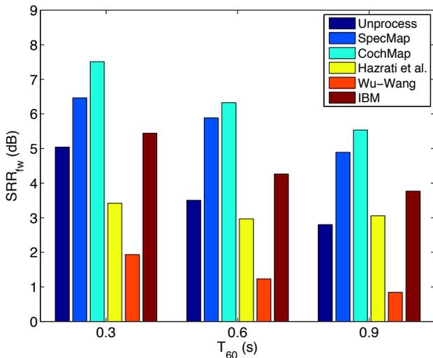
**Fig. 3:**  $SRR_{fw}$  comparisons. “Unprocess” denotes the  $SRR_{fw}$  results for unprocessed reverberant speech. “SpecMap” and “CochMap” denote the proposed spectral mapping approach using spectrogram and cochleagram, respectively. “Hazrati et al.”, “Wu-Wang”, and “IBM” denote three baselines as described.
