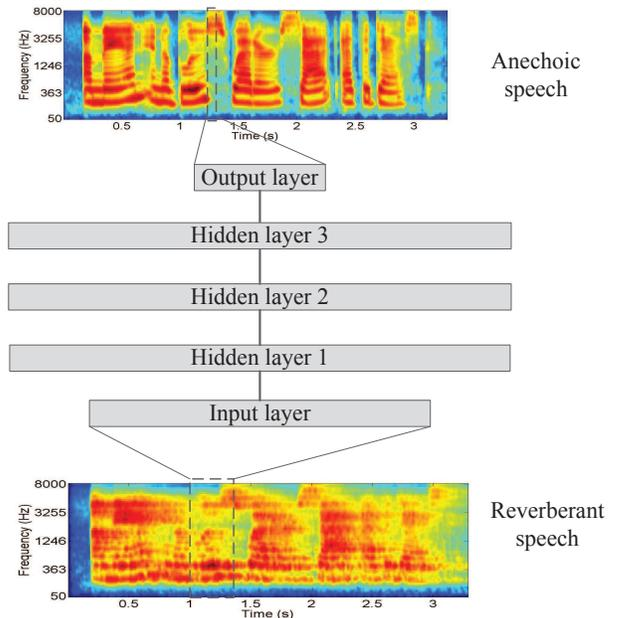
Fig. 1: Structure of the DNN for dereverberation.
