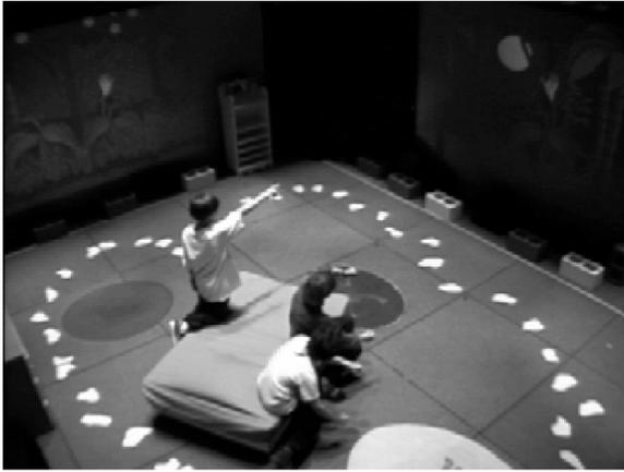
Fig. 9. The KIDSRROOM interactive play-space. Using a modified version of temporal templates, the room responds to the movements of the children. All sensing is performed using vision from three cameras: one overhead for tracking and two wall mounted cameras for movement recognition.
