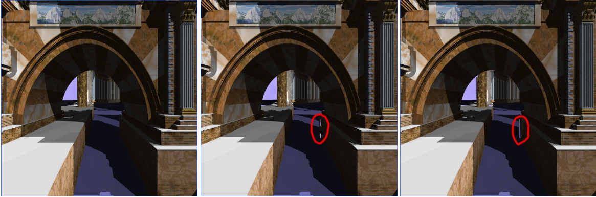
Figure 5. Shows the rendering images with track dependent occlusion culling with \alpha values equal to 1, 0.9 and 0.8 respectively. Notice the artifacts indicated by the red circle when decreasing the \alpha threshold.
