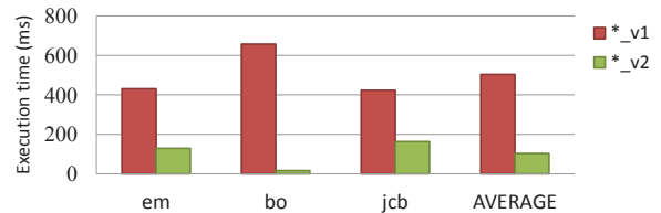
Figure 5: Performance improvement from tuning the use of GPU memory hierarchy based on GMProf’s profiled data.
